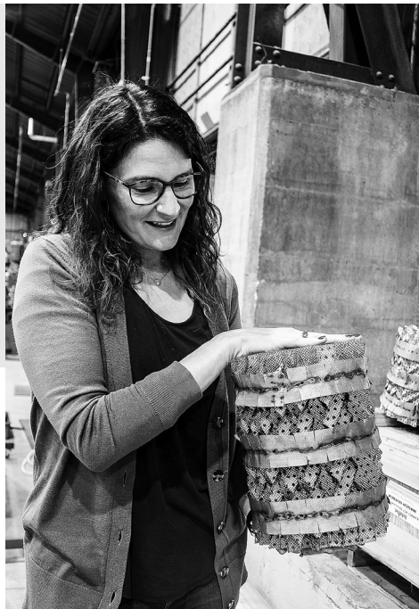
Courtney McKee with a distillation column internal used in the distilling process at Headframe Spirits.
